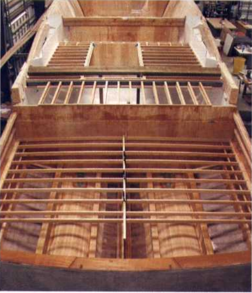
Whiticar's new 76-foot sportfishing yacht in various stages of completion: (Top left) The keel plate consists of epoxy-laminated mahogany planking that runs the full length of the boat. The individual planks are clamped and glued together on the hull jig and become a continuous backbone for the vessel. (Top right) One layer of diagonally planked mahogany used on the hull sides. The next two layers of planking will be installed in the opposite angles, creating a hull side with strength in multiple directions. (Center) Rendering of the completed yacht. (Bottom left) The hull is constructed upside down over a removable computer-routed jig. When the basic hull is completed, the jig is removed and the boat is rolled outside and flipped over. Many of the deck beams and structural components can be installed inside the boat prior to flipping over. (Bottom right) Breaking tradition on the new 76 model, Whiticar has switched over from a deckhouse constructed completely out of wood to a modern fiberglass-and-foam composite structure. A composite house yields a stronger and lighter part and also allows improved stylings, which are more difficult to create out of wood. PHOTOS COURTESY OF WHITICAR CUSTOM BOATS
