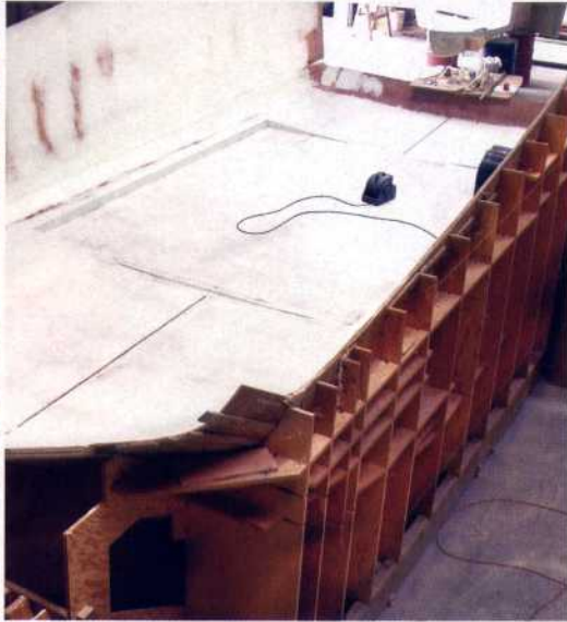
Whiticar's new 76-foot sportfishing yacht in various stages of completion: (Top left) The keel plate consists of epoxy-laminated mahogany planking that runs the full length of the boat. The individual planks are clamped and glued together on the hull jig and become a continuous backbone for the vessel. (Top right) One layer of diagonally planked mahogany used on the hull sides. The next two layers of planking will be installed in the opposite angles, creating a hull side with strength in multiple directions. (Center) Rendering of the completed yacht. (Bottom left) The hull is constructed upside down over a removable computer-routed jig. When the basic hull is completed, the jig is removed and the boat is rolled outside and flipped over. Many of the deck beams and structural components can be installed inside the boat prior to flipping over. (Bottom right) Breaking tradition on the new 76 model, Whiticar has switched over from a deckhouse constructed completely out of wood to a modern fiberglass-and-foam composite structure. A composite house yields a stronger and lighter part and also allows improved stylings, which are more difficult to create out of wood. PHOTOS COURTESY OF WHITICAR CUSTOM BOATS
